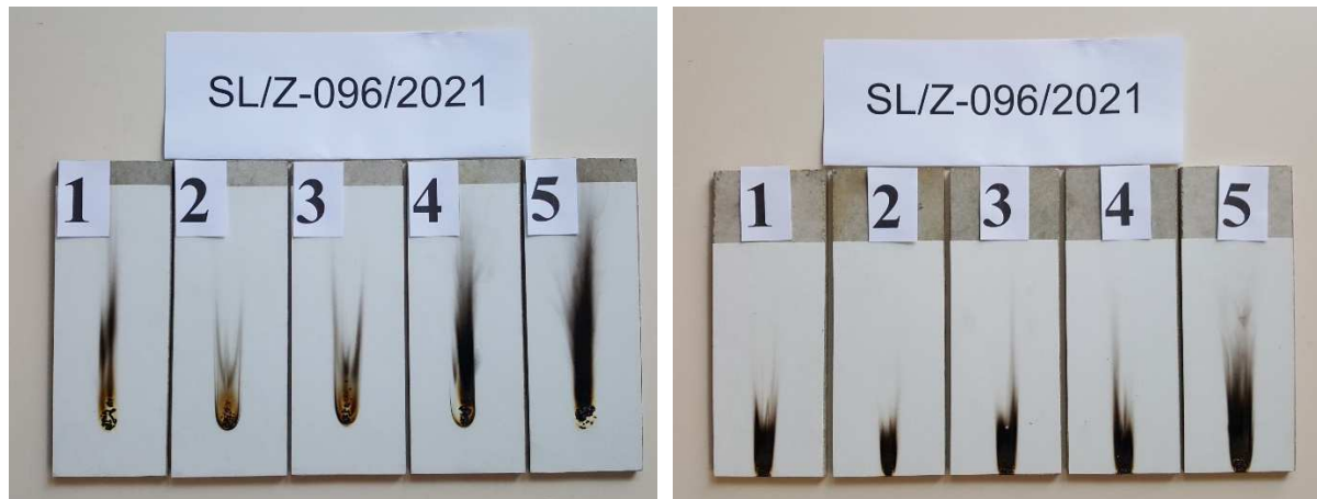
Figure 5. Appearance of the specimens after the small burner test
